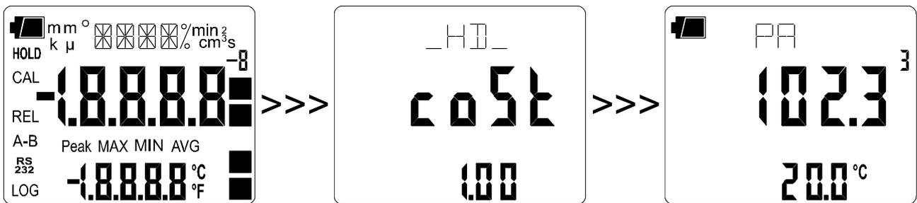
If no thermocouple probe is connected to the input, it is the manual temperature which is displayed in the secondary line. This value is 25°C by default.
