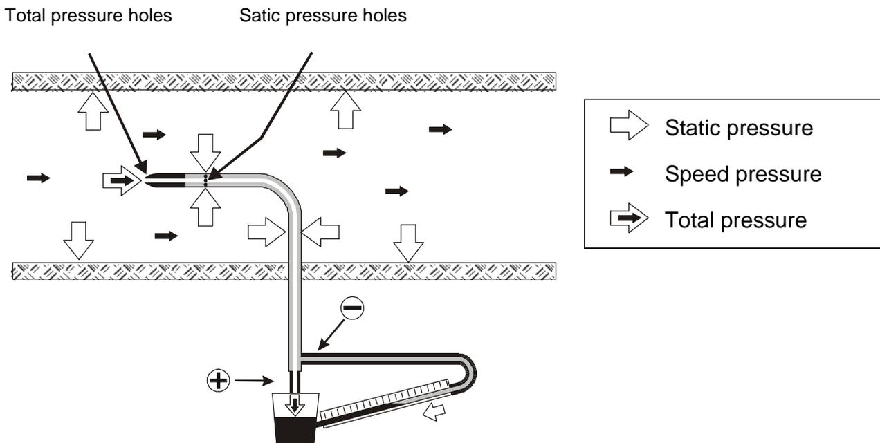
The pressure inside the duct is the result of three different pressures:
