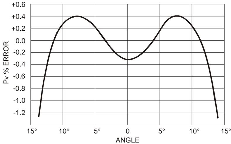
The abscissas reports the rotation angle around its vertical axis compared to the flow direction (yawing), in ordinates the % error on the differential pressure Pv measurement. As you can see a difference of over 10° entails an error on the differential pressure Pv measurement of less than 0.5%.
