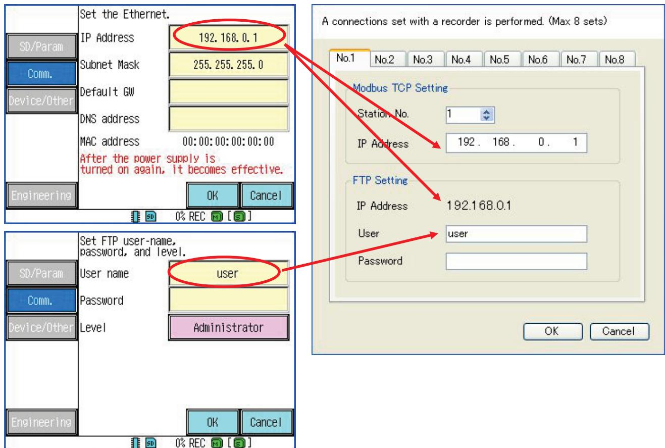
The “IP Address” of “Modbus TCP Setting” and “FTP Setting” is set to become it as well as “Paperless recorder (※Ethernet1)”. (In this case, “IP Address” is set as “192.168.0.1”).
