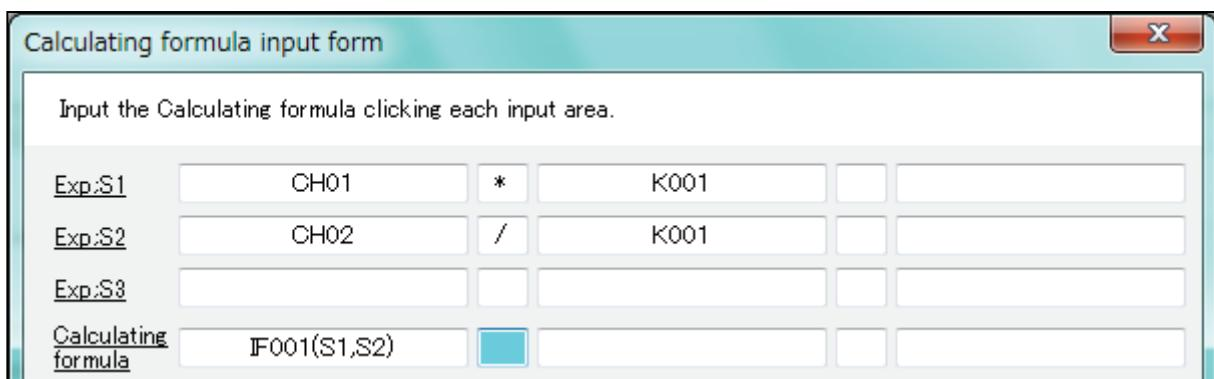
If set up as mentioned above. When the value of CH01 is larger than the value of CH02, the argument A of conditional branch IF001 (Exp; S1) is outputted to CH13. Moreover, when the value of CH01 is equal or smaller than the value of CH02, the argument B of conditional branch IF001 (Exp; S2) is outputted to CH13.
