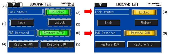
When [Lock] is pressed. When RUN after power restoration is selected.
