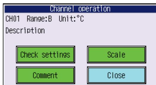
**Check settings** : The setting status can be verified. And, a set item that becomes an object is selected touching, and **Change set** key can be moved directly to the selected set screen by touching.
