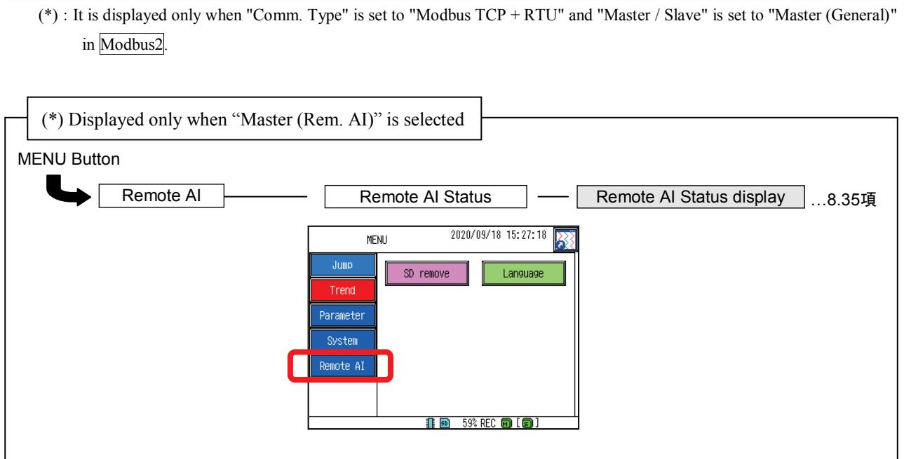
(\*) : It is displayed only when "Comm. Type" is set to "Modbus TCP + RTU" and "Master / Slave" is set to "Master (Rem. AI)" in Modbus2.
