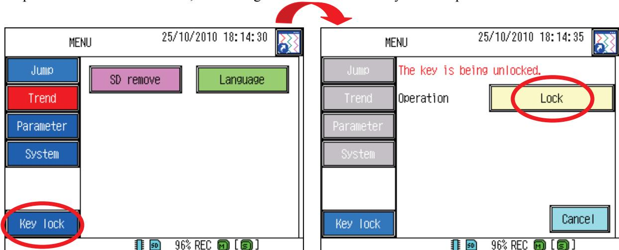
If a key lock is set up, a limit as shown in the following figure is performed to a menu screen and a hard key.
