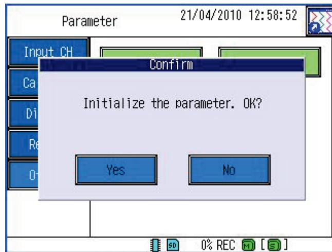
When [Param initial] key is selected, the confirmation screen (above figure) is displayed. The parameter data is initialized when selecting [YES] key.
