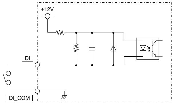
No-voltage contact input (9 point), terminals (DI\_COM) of each channel are common.
