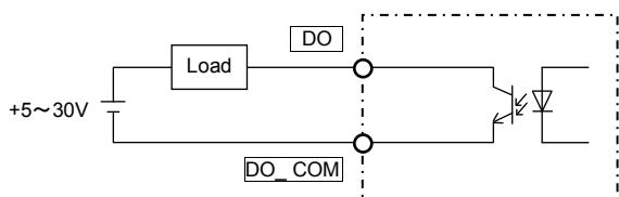
Open collector output (12 point) , terminals (DO\_COM) of each channel are common.
