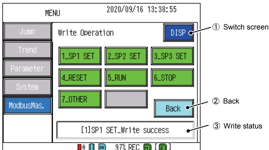
On this screen, the button with the button name set in "Wrt (Display) " in Section 8.29 is displayed.
