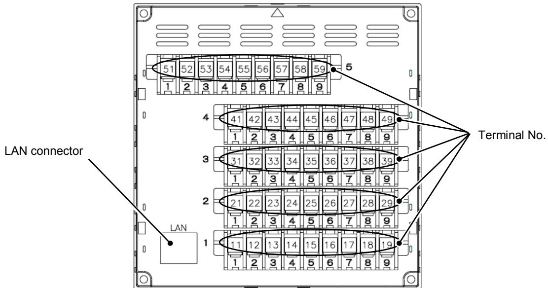
**Fig. 4-1 Terminal stand array(The back of recorder)**
