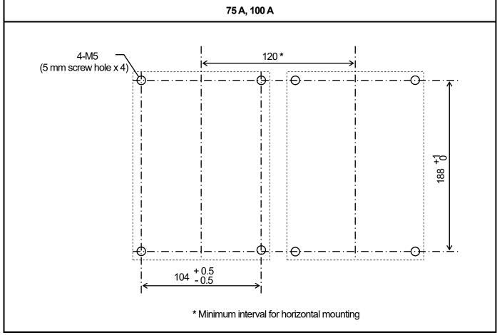
Note: Keep space for heat radiation of more than 200 mm above and below this unit.
