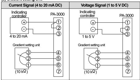
(4) Manual setting unit with gradient setting unit
