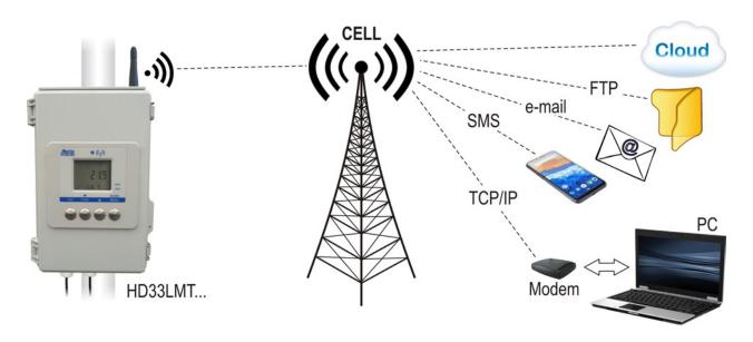
The data logger can be controlled remotely either by sending commands via SMS messages or by establishing a direct TCP/IP connection via mobile network with a remote PC connected to the Internet.
