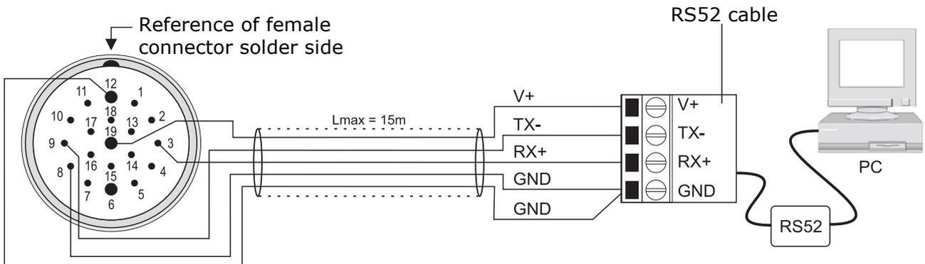
To use the **RS52** cable, the drivers included in the HD52.3D-S software package should be installed in the PC (see the guide to USB drivers installation included in the software package).
