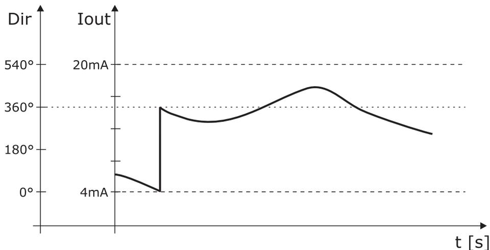
If 539° value is exceeded in extended mode, the output goes to the value corresponding to 180°. The table below shows the correspondence between the value of the analog output and the direction of the wind in the two modes.
