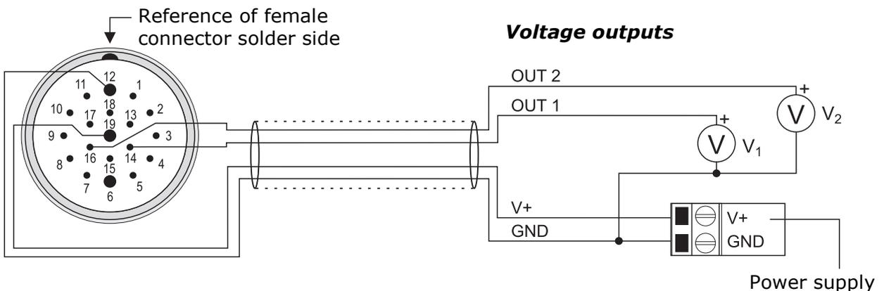
Load resistance:  $R_L > 10 \text{ k}\Omega$ .
