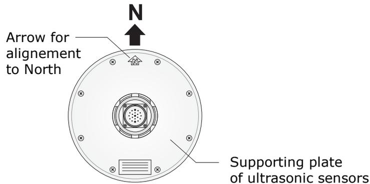
For an accurate alignment, connect the instrument to a PC (see following chapters for communication protocols), then rotate the instrument on its vertical axis until the compass measures  $0.0^\circ \pm 0.1^\circ$ .
