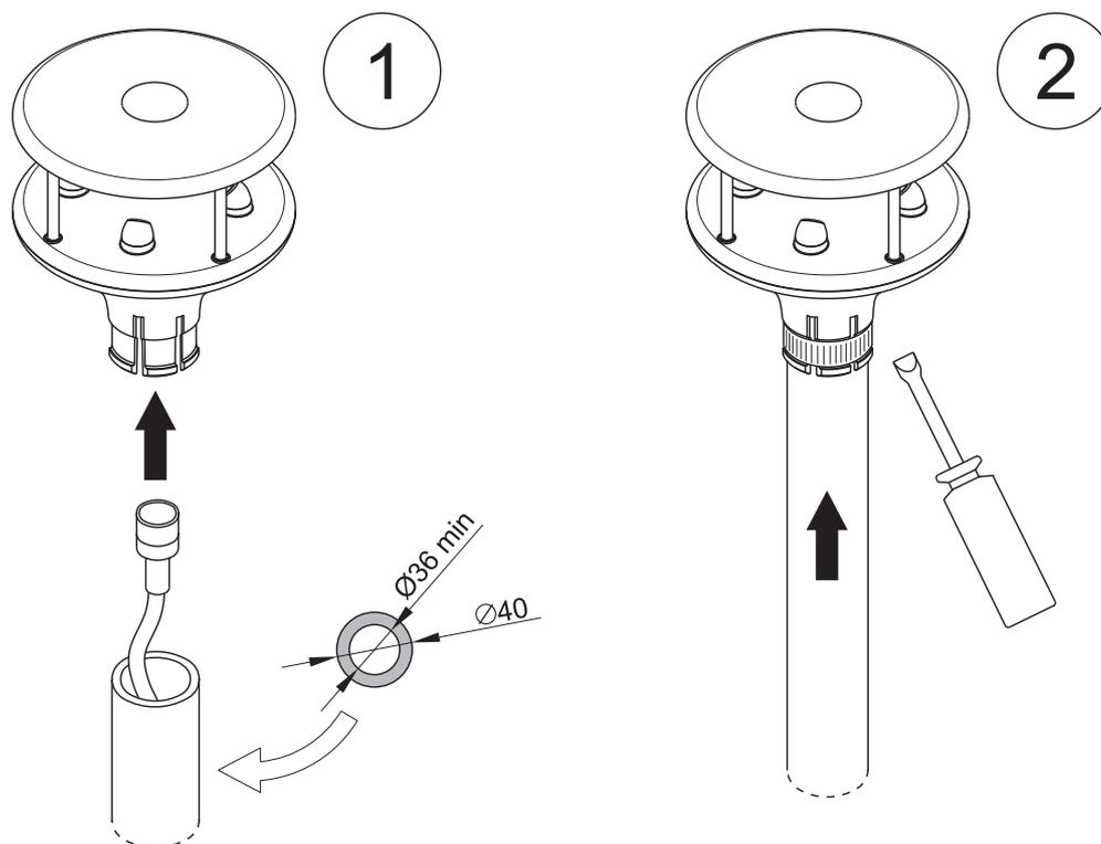
The support mast, having 40 mm maximum outer diameter and 36 mm minimum inner diameter, should be positioned on a stable surface.
