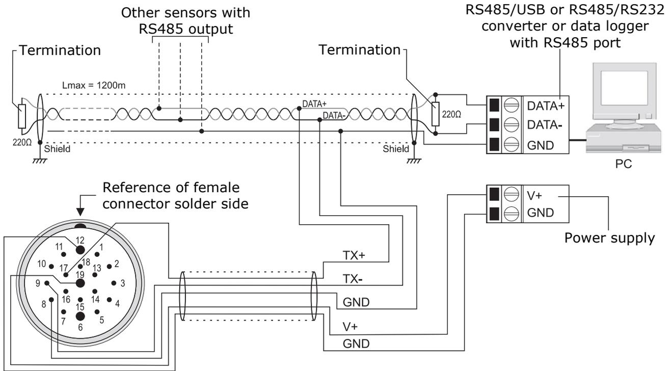
Thanks to RS485 connection, multiple instruments can be connected to a multi-point network. Instruments are connected in sequence through a twisted-pair shielded cable for signals and a third wire for ground.
