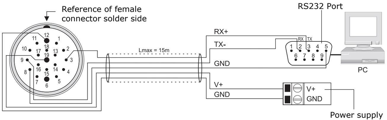
For RS232 connection, TX-, RX+ and serial GND signals (pin 9, 3 and 8 of M23 connector) are used, to be connected respectively to RX, TX and GND signals of RS232 port on PC (pin 2, 3 and 5 of 9-pole SubD connector). The length of RS232 cables should not exceed 15 m.
