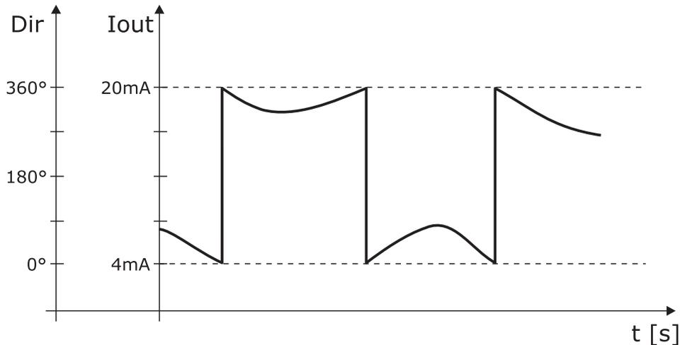
This effect can be reduced through the extended ("wrap-around") characteristic of wind direction. In this mode, the wind direction is considered as corresponding to 0÷539° range instead of 0÷359°. The wide output fluctuation occurs the first time that the wind direction goes from 0 to 359°; if later the "physical" direction goes back to 0°, the analog output will always remain around 360°. Using the extended characteristic, the behavior of the above graph changes into the following:
