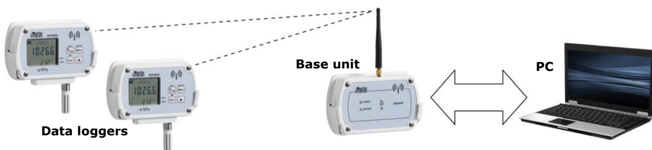
Fig. 2.1: base unit placed between data loggers and PC
