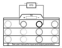
Figure 16 Simulate RTD Output
