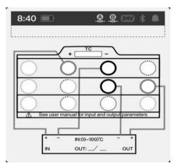
Figure 20 Temperature switch
