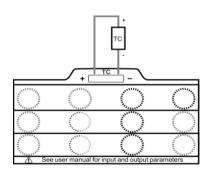
Figure 8 Thermocouple measurement
