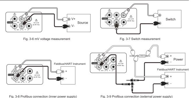
Fig. 3-9 Profibus connection (external power supply)
