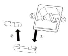
Figure 7-3 Diagram of Fuse Replacement
