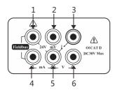
Fig. 3-3 Electric signal measurement terminal diagram
