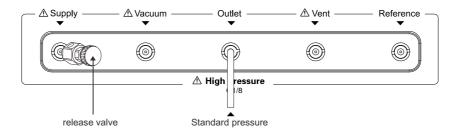
Fig 7-1 Connection of External Standard Pressure
