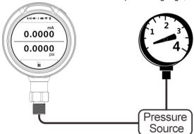
Figure 12 Calibrate Dial Pressure Gauge
