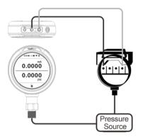
Figure 13 Calibrate pressure transmitter
