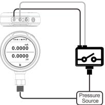
Figure14 Calibrate Pressure Switch
