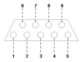
Figure 18 Description of RS232 module DB9 female pins
