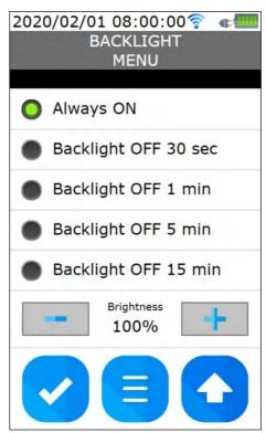
Use the  $\pm$ - keys to adjust the display brightness. The lower the display brightness, the longer the battery autonomy will be.
