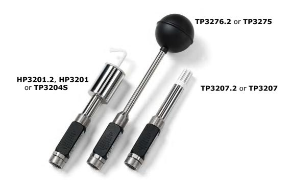
Probes necessary for **PMV/PPD** indices measurement:
