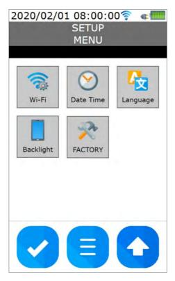
The FACTORY sub-menu includes advanced system functions for the technical maintenance of the instrument and is accessible after entering a numeric password.
