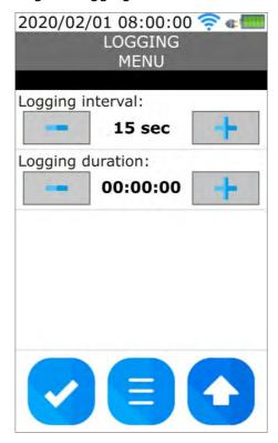
Use the +/- keys to change the interval an to set any logging duration.
