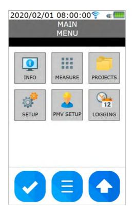
**INFO**: instrument and connected probes general information. **MEASURE**: choice of the measurement screens to be displayed.
