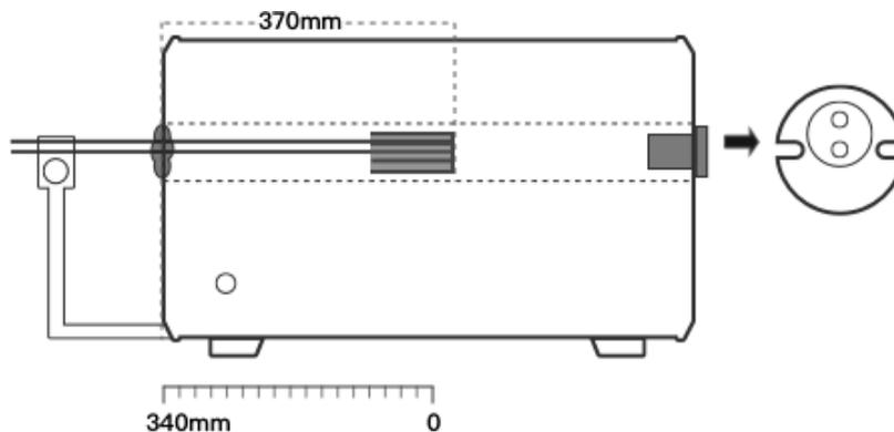
Figure 2-9 Base metal + long furnace + multi-hole insert
