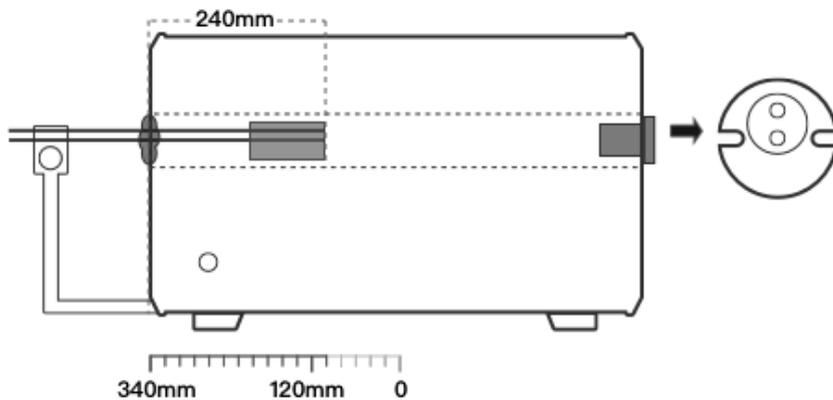
Figure 2-12 Base metal + short furnace + cup design insert
