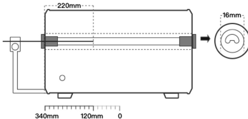
Figure 2-14 Noble metal +  $\phi 16\text{mm}$  alumina tube
