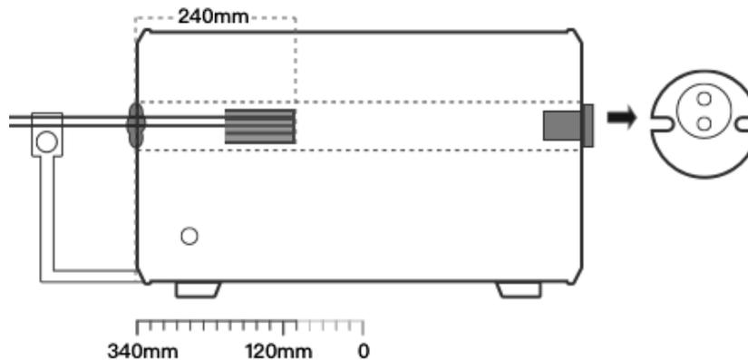
Figure 2-13 Base metal + short furnace + multi-hole design insert
