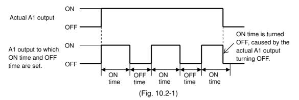
A output status can be read by reading Status flag 2 (A11, A12, A21, A22 output flag bit) in Serial communication.
