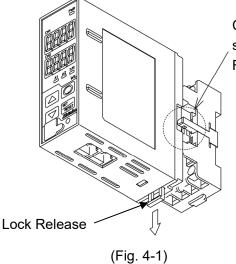
Check that the WIL-102-ECL and the socket are unlocked by pulling the Lock Release down.
