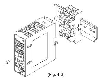
(4) Remove the socket from the DIN rail by pulling the socket Lock Release (at the bottom of the socket) down.
