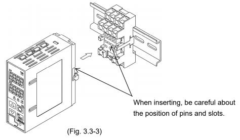
(4) Fix the WIL-102-ECL and the socket by pushing the Lock Release up.
