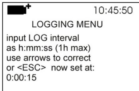
1. Use the arrows **▲ ▼** to select the interval duration from **a minimum of 2 seconds to a maximum of one hour**;
