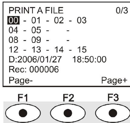
1. Use the arrows ▲▼◀▶ to select the log to be printed, and the F1 and F3 function keys to shift page.
