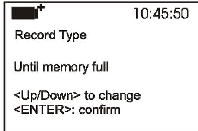
The memory can be handled in two modes that can be selected using the ▲▼ arrows:
