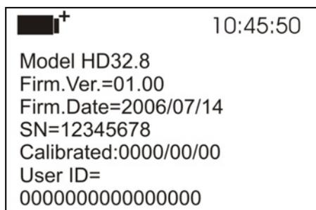
This screen cannot be modified: The user identification code (User ID) can be set using the DeltaLog9 software.
