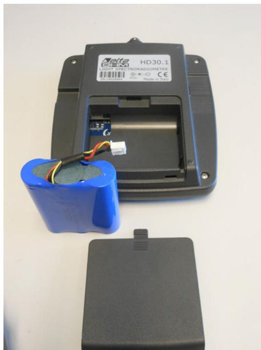
*Figure 2.2: Battery removed from housing.*
