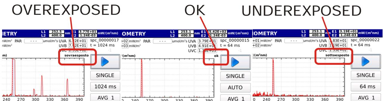
Fig. 3.24: The correct exposure is indicated on top of the graph.
