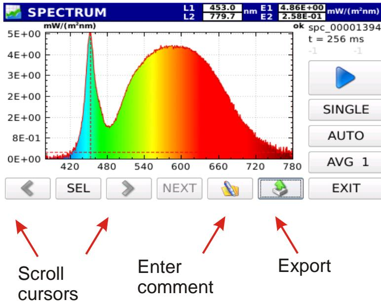
Figure 3.7: Spectrum display at the end of measurement
