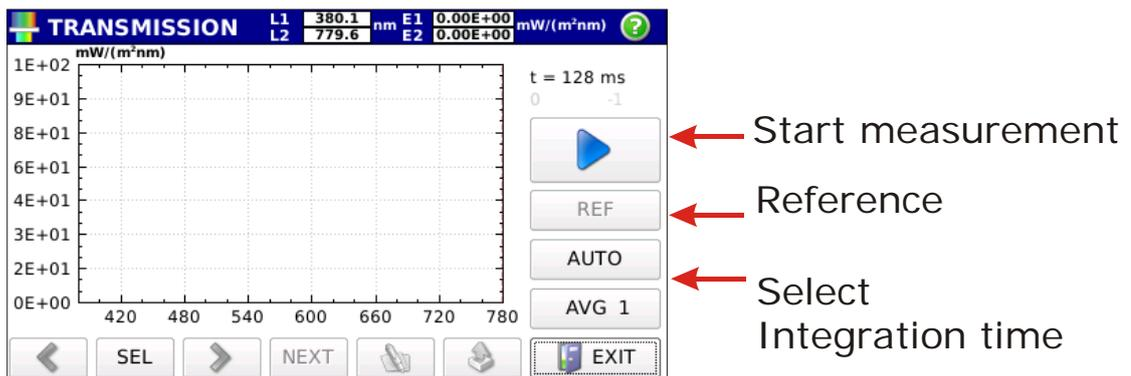
Fig. 3.23: Transmission measurement screen
