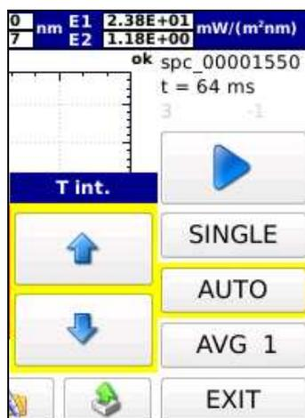
3.3.2.1 **Manual Selection:** the integration time can be manually selected by using
