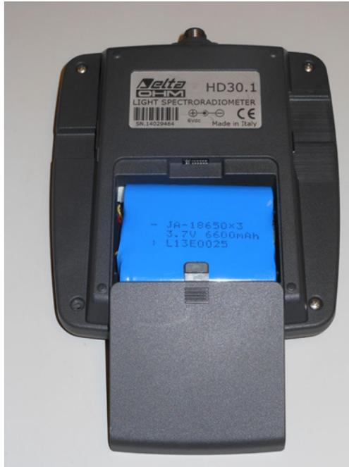
*Figure 2.1: Disconnected battery inside battery compartment.*
