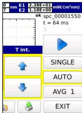
**3.4.2.1 Manual selection:** the integration time is manually selected using the arrows
