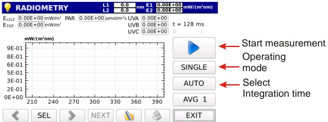
Fig3.17 Start-up screen in radiometry mode
