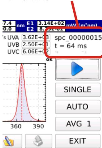
Fig. 3.21: File name and integration time data are shown on top right of the screen
