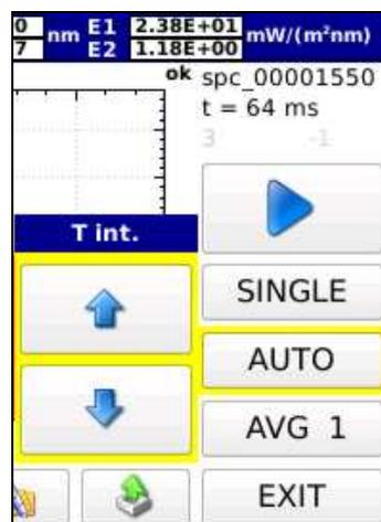
3.2.2.1 **Manual Selection:** the integration time is selected manually by using the arrow
