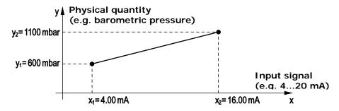
Fig. 13.6.1: example of association of a physical quantity to the acquired signal
