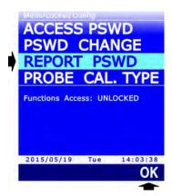
4. Set the first digit using the password with ▲ and ▼, then select the "-->" command (F2 key) to move to the next digits (the currently selected digit flashes). To return to a previous digit, select the "<--" command (F1 key). After setting all the digits, press OK (F3 key) to confirm the new password.</p>
