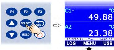
2. Select the **SETUP** item using ▲ and ▼, then press the **F3** key (**OK** command) to confirm.
