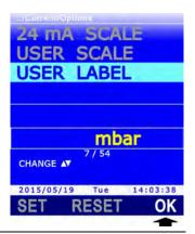
3. To define a new unit, select "....." item using ▲ and ▼, then press the F1 key (command SET) to confirm.
