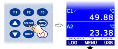
2. Select the **CALIBRATION** item using ▲ and ▼, then press the **F3** key (**OK** command) to confirm.
