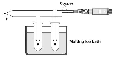
Fig. 4.2.1: cold junction at 0 °C
