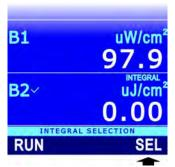
4. The indication INTEGRAL over the measurement unit is replaced by the integration countdown, to indicate that the measurement line is selected for calculating the integral.
