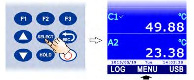
2. Select the **LOCKED CONFIG** item using ▲ and ▼, then press the **F3** key (**OK** command) to confirm.
