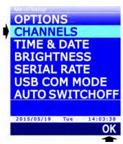
6. Using ▲ and ▼, select the input (A, B or C) of the instrument to which the probe is connected, then press F3 (OK command) to confirm.
