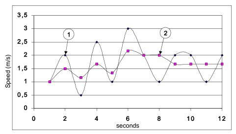
Fig. 9.5.1: average effect in air speed measurements
