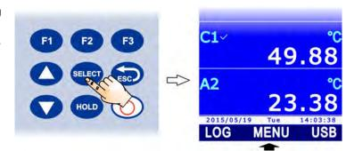
2. Select the **LOCKED CONFIG** item using ▲ and ▼, then press the **F3** key (**OK** command) to confirm.
