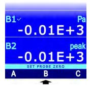
Fig. 4.4.2: selecting the differential probe for zeroing
