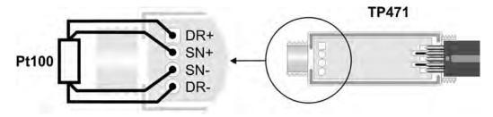
Fig. 4.1.2: connecting 4-wire Pt100 sensor to TP471 module
