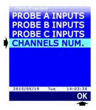
2. Set the number of measurement lines to be displayed using ▲ and ▼ (select the RESET command with F2 key to set the default number), then press F3 (OK command) to confirm.
