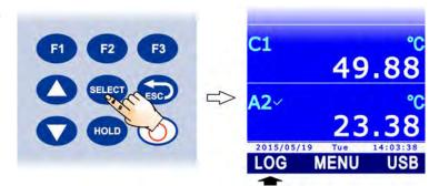
2. To start logging, select the **RUN** command by pressing the **F1** key.
