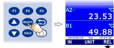
3. The selected measurement line shows the difference between the quantity current value and the reference value, consisting in the measurement value at the moment of the REL command activation. The reference value is displayed in the upper part of the measurement line (followed by the symbol REL).
