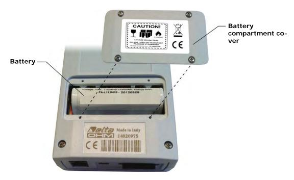
Fig. 12.2: battery compartment
