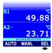
4. The indication "0 rcd" appears on the upper part of the measurement line, to indicate that the quantity has been selected for the RECORD function.
