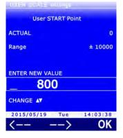
6. Set the maximum value of the physical quantity to be associated to the voltage or current values (e.g. 1100, point Y2 of the example at Fig. 13.6.1). Set the first digit using ▲ and ▼, then select the "-->" command (F2 key) to move to the next digits (the currently selected digit flashes). To return to a previous digit, select the "<--" command (F1 key). After setting all the digits, press OK (F3 key) to confirm the value.</p>
