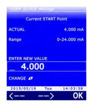
4. Set the maximum value of the voltage or current signal (e.g. 16 mA, point X2 of the example at Fig. 13.6.1). Set the first digit using ▲ e ▼, then select the "-->" command (F2 key) to move to the next digits (the currently selected digit flashes). To return to a previous digit, select the "<--" command (F1 key). After setting all the digits, press OK (F3 key) to confirm the value.</p>
