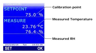
Fig. 13.3.5: calibration at 75%RH
