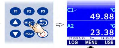
3. If necessary, select the **HELP** item using ▲ and ▼ keys, then press **F3** key (OK command) to confirm.
