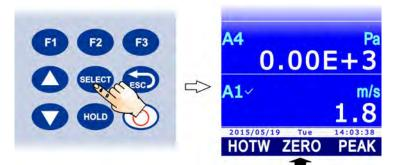
3. Select **A**, **B** or **C** input the probe is connected to by pressing **F1**, **F2** or **F3** key respectively.
