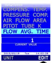
6. Set the first digit using ▲ and ▼, then select the "-->" command (F2 key) to move to the next digits (the currently selected digit flashes). To return to a previous digit, select the "<--" command (F1 key). After setting all the digits, press OK (F3 key) to confirm the value.</p>
