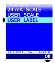
2. Using ▲ and ▼, select a measurement unit (e.g. mbar) for the physical quantity to associate to the voltage or current values, then press the F3 key (OK command) to confirm. If the measurement unit is not available among the listed units, you can select the generic item user or define a new unit. Proceed to the next step to define a new unit.
