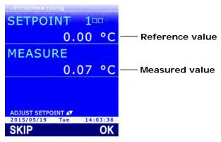
Fig. 13.1.2: PRT calibration at 0 °C
