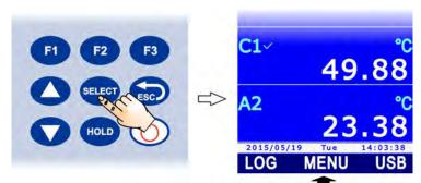
2. Select the **LOG SETTINGS** item using ▲ and ▼, then press the **F3** key (**OK** command) to confirm.
