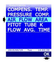
5. The section current setting appears. Select the **UNIT** command by pressing the **F1** key to change the measurement unit (cm<sup>2</sup> or in<sup>2</sup>).
