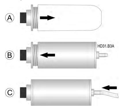
Fig. 13.5.3: CO<sub>2</sub> calibration with nitrogen bottle
