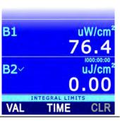
4. Set the first digit using ▲ and ▼, then select the command "-->" (F2 key) to move to the next digits (the currently selected digit flashes). To return to a previous digit, select the command "<--" (F1 key). After setting all the digits, press OK (F3 key) to confirm the value.</p>
