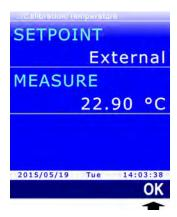
Fig. 13.3.3: calibration of the Pt100 sensor to the reference value
