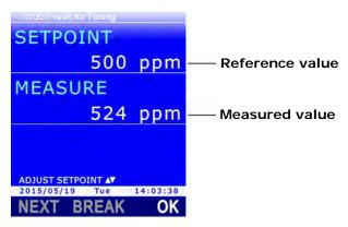
Fig. 13.5.2: ZERO/FRESH AIR calibration for CO2 probes
