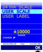
3. Set the minimum value of the voltage or current signal (e.g. 4 mA, point X1 of the example at Fig. 13.6.1). Set the first digit using ▲ and ▼, then select the "-->" command (F2 key) to move to the next digits (the currently selected digit flashes). To return to a previous digit, select the "<--" command (F1 key). After setting all the digits, press OK (F3 key) to confirm the value.
