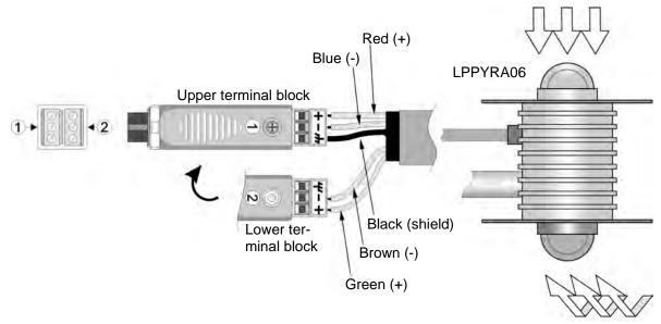
Fig. 4.6.3: connecting LPPYRA06 albedometer
