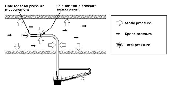
Fig. 4.5.9: Pitot tube measuring principle
