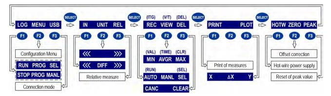
Fig. 2.3.1: functions in the command bar
