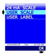
2. Using ▲ and ▼, select a range (e.g. ±10000) for the physical quantity to be associated to the voltage or current values, then press the F3 key (OK command) to confirm.
