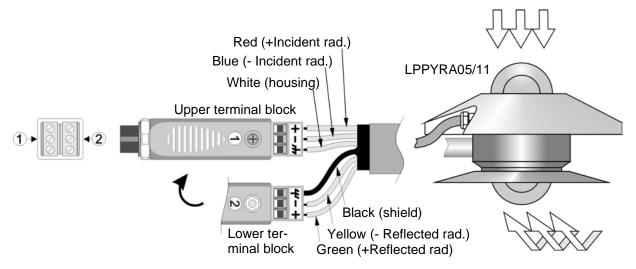
Fig. 4.6.2: connecting LPPYRA05 and LPPYRA11 albedometers
