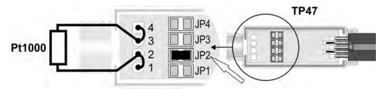
Fig. 4.1.4: connecting 2-wire Pt1000 sensor to TP47 connector
