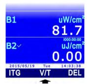
3. Select **TIME** (**F2** key) to set the integration time limit, or **VAL** (**F1** key) to set the threshold limit of the integral.
