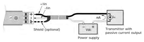
Fig. 4.9.3: IP472 module connected to transmitter with passive current output
