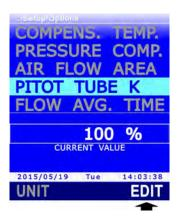
6. Set the first digit using ▲ and ▼, then select the "-->" command (F2 key) to move to the next digits (the currently selected digit flashes). To return to a previous digit, select the "<--" command (F1 key). After setting all the digits, press OK (F3 key) to confirm the value.
