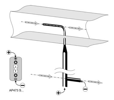
Fig. 4.5.10: positioning the Pitot tube
