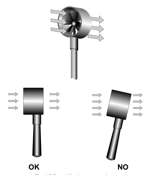
Fig. 4.5.7: positioning vane probes
