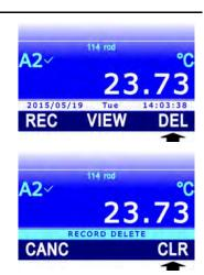
To disable the RECORD function, select instead the **CANC** command by pressing the F1 key. Press **ESC** to return to the previous menu level.
