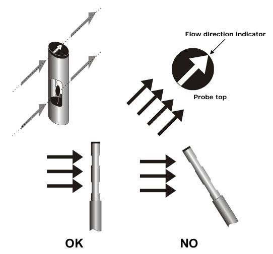
Fig. 4.5.4: positioning hot wire probes
