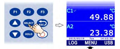
2. Select the **LOG SETTINGS** item using ▲ and ▼, then press the **F3** key (**OK** command) to confirm.
