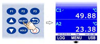
2. Select the **LOCKED CONFIG** item using ▲ and ▼, then press the **F3** key (**OK** command) to confirm.
