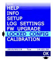
3. The current protection status (Access Functions) appears at the end of the menu item list. The word LOCKED indicates the protected status; the word UNLOCKED indicates the unprotected status. To change the status, select the ACCESS PSWD item, using ▲ and ▼ if necessary, then press the F3 key (OK command) to confirm.
