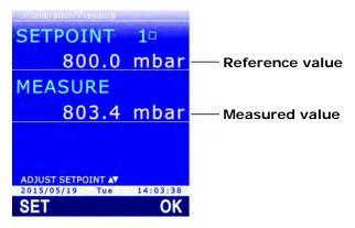
Fig. 13.4.1: barometric pressure calibration
