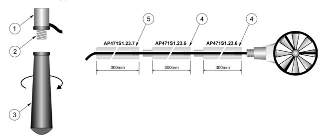
Fig. 4.5.8: adding extensions to vane probes
