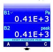
Fig. 4.4.4: selecting the probe for peak value reset
