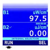
The RUN command starts the integral of all the INTEGRAL-type measurements selected for calculation. If integral measurements have not been specifically selected, the integral of all the INTEGRAL-type measurements is started.
