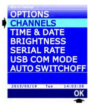
4. Select the A, B or C input of the instrument, using ▲ and ▼, then press F3 (OK command) to confirm.
