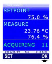
Fig. 13.3.6: calibration point confirmation
