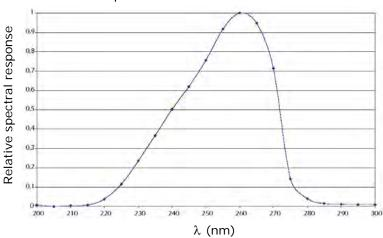
**LP471UVBC** Probe for the measurement of **UVBC irradiance**, with SICRAM module.
