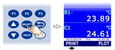
Select the PRINT command by pressing the F1 key, the information regarding the connected probes (type of probe, serial number and type of calibration) and the three measurements currently displayed are sent to the printer or to the PC.
