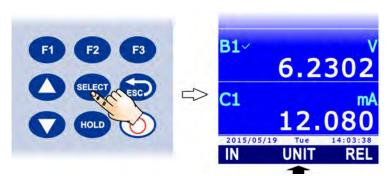
3. Select "<<<" (**F1** key) or ">>>" (**F3** key) to move from the voltage or current value to the associated physical quantity.
