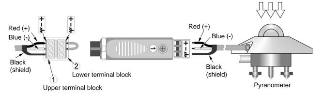
Fig. 4.6.1: connecting a pyranometer
