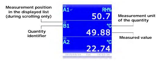
Fig. 3.2: measurements display
