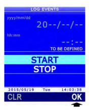
4. Select the different date/time fields using "<<<" (**F1** key) or ">>>" (**F2** key) commands, the selected field flashes. Use ▲ and ▼ to change the value.
