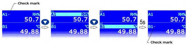
Fig. 3.1.1: selecting a measurement line
