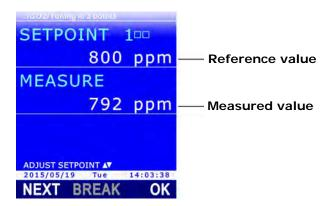
Fig. 13.5.5: LINEAR GAINS calibration for CO<sub>2</sub> probes
