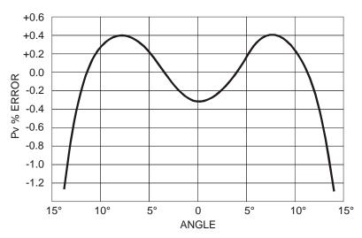
Fig. 4.5.11: misalignment error of the Pitot tube
