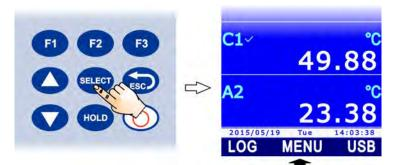
Select the SETUP item using ▲ and ▼, then press the F3 key (OK command) to confirm.
