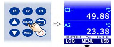
2. Select the **SETUP** item using ▲ and ▼, then press the **F3** key (**OK** command) to confirm.
