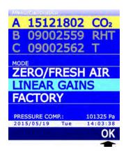
Fig. 13.5.1: calibrations for CO<sub>2</sub> probes
