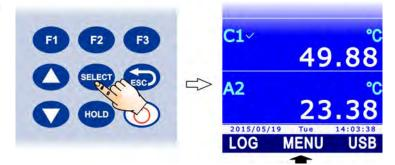
4. Select the **SETUP** item using ▲ and ▼, then press **F3** (**OK** command) to confirm.
