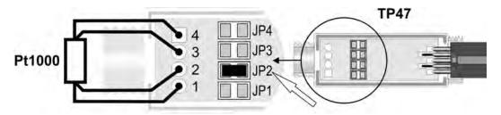
Fig. 4.1.5: connecting 4-wire Pt1000 sensor to TP47 connector
