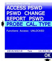
4. Select the probe connected to A, B or C input using the **PROBE** command (**F1** key).
