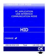
5. The instrument returns to the USB COM MODE item, press **ESC** twice to exit the menu.
