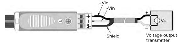
Fig. 4.9.1: VP473 module connected to voltage output transmitter
