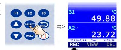
2. Select the **AUTO** command by pressing **F1** to start automatic once-per-second sample acquisition.
