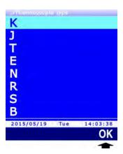
Fig. 13.2.1: selecting the type of thermocouple
