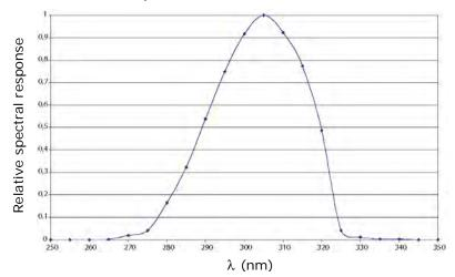
**LP471UVC** Probe for the measurement of **UVC irradiance**, with SICRAM module.
