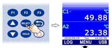
2. Select the **LOCKED CONFIG** item by using ▲ and ▼, then press the **F3** key (**OK** command) to confirm.
