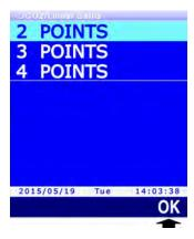
Fig. 13.5.4: CO<sub>2</sub> multi-point calibration
