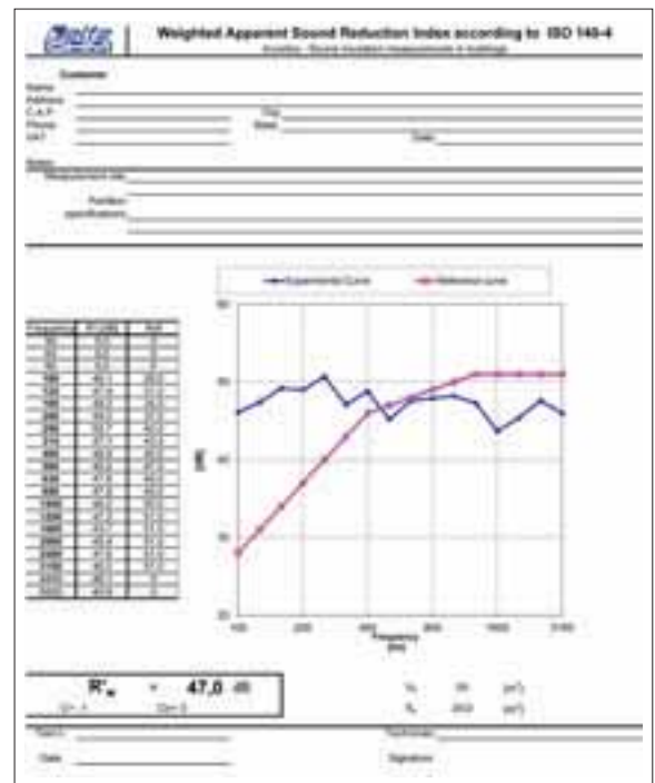
Noise Studio: NS3 "Acoustic Insulation" module; ISO717 report.
