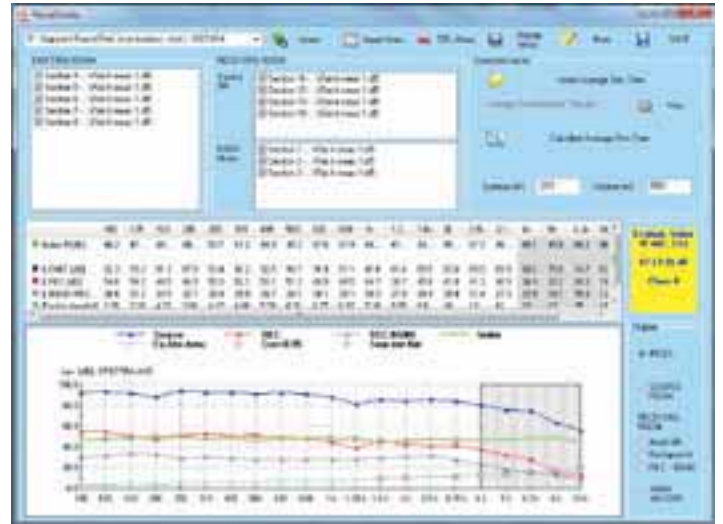
Noise Studio: NS3 "Acoustic Insulation" module; calculation of airborne sound insulation and impact noise descriptors.
