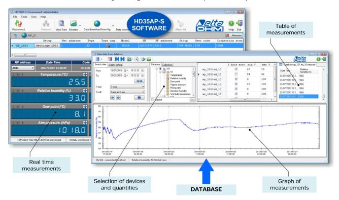
The database functions allow viewing the data coming from multiple data loggers simultaneously. The connection to the database is **multi-client**: it is possible to store the data in a remote database on the local network to which the PC is connected, and the data can be viewed from any PC on the network via the HD35AP-S software.
